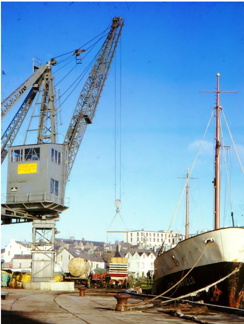
The MV Fallowfield moored at Portrush prior to her final sailing. The 25-ton Butters crane which dominated the harbour landscape during the operation of the Portrush-Preston service, was dismantled not long afterwards.
